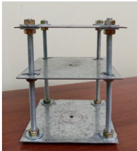
Figure1 hand-made tool use to espouse the detector with different energy by changing the distances between the source and the detector.
